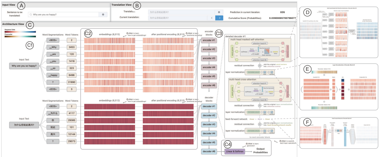
Fig. 1: With TransforLearn, learners can gain an understanding of the Transformer structure and the process of machine translation. Input view (A) provides an interface for the text to be translated. Translation view (B) displays the model’s translation results and current translation progress, helping users in task-driven exploration. Architecture view (C) provides an overview of the visualized model structure and data flow, with sub-views (C1-C4) that support the close exploration of computational processes. Once enabled, the detailed view (C3) displays the attention mechanism view (D), layer normalization view (E), and feed-forward network view (F). These views not only show the data flow and operational details but also support multiple interactions.
